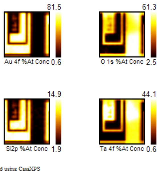
Figure 11: Si 2p image is enhanced using a PCA reconstruction technique based on Optimum Scaling.
